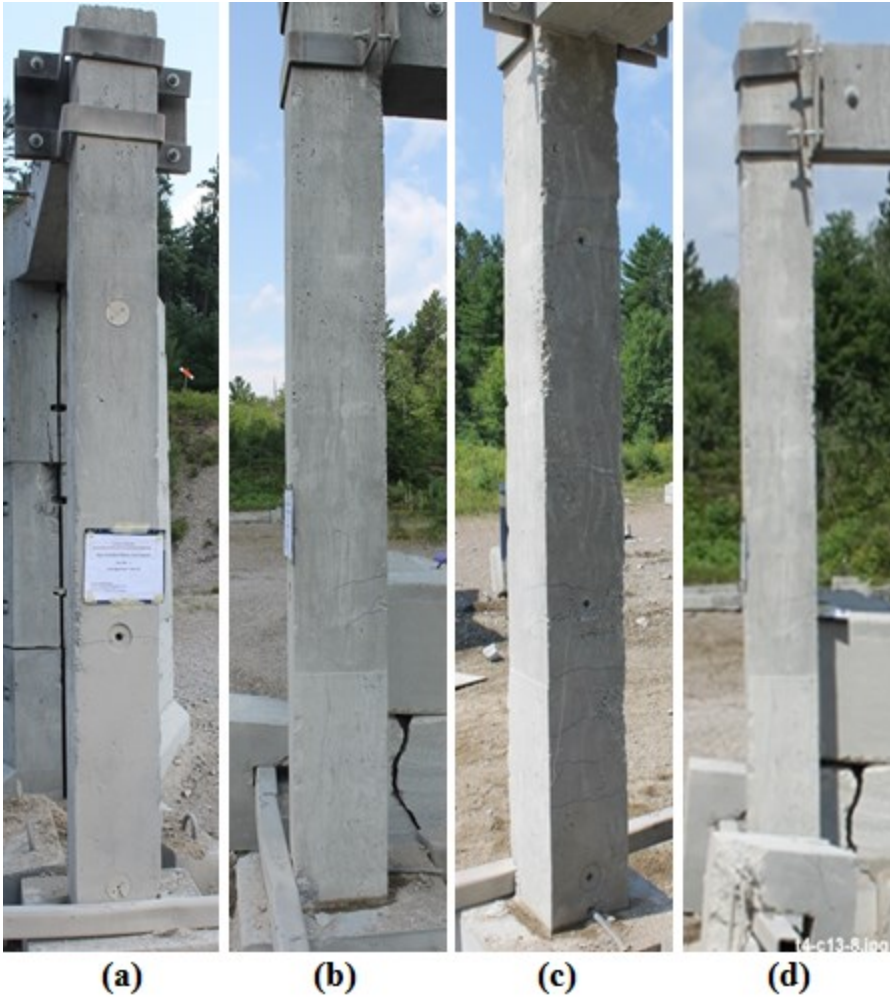
Figure 4-47: Post-test photograph of Column SEIS-13 faces: (a) Front face, (b) and (d) Side face (right), and (c) Back face
