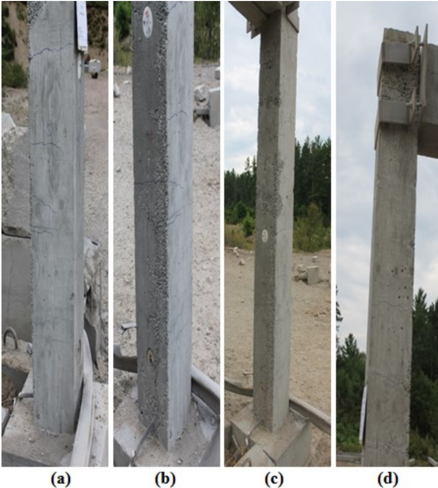
Figure 4-58: Post-test photograph of Column SEIS-11 face: (a) Side face (right), (b, c) Back face, and (d) Side face (left)
