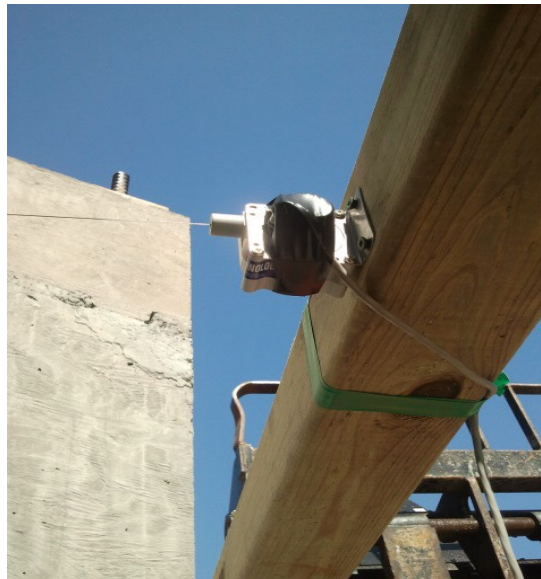
Figure 3-23: Transducer mount on 89×89 mm wood stud
