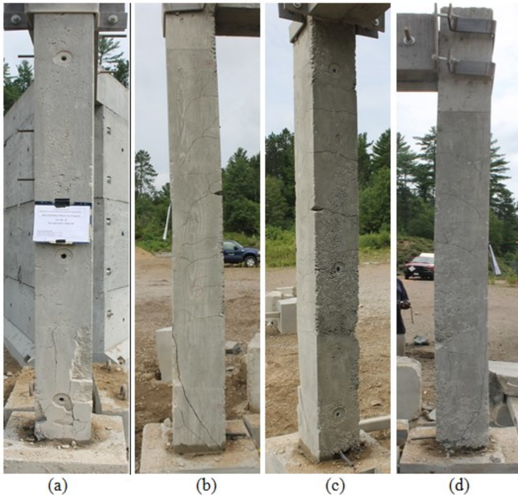
Figure 4-35: Post-test photograph of Column CONV-6 faces: (a) Front face, (b) Side face (right), (c) Back face, and (d) Side face (left)
