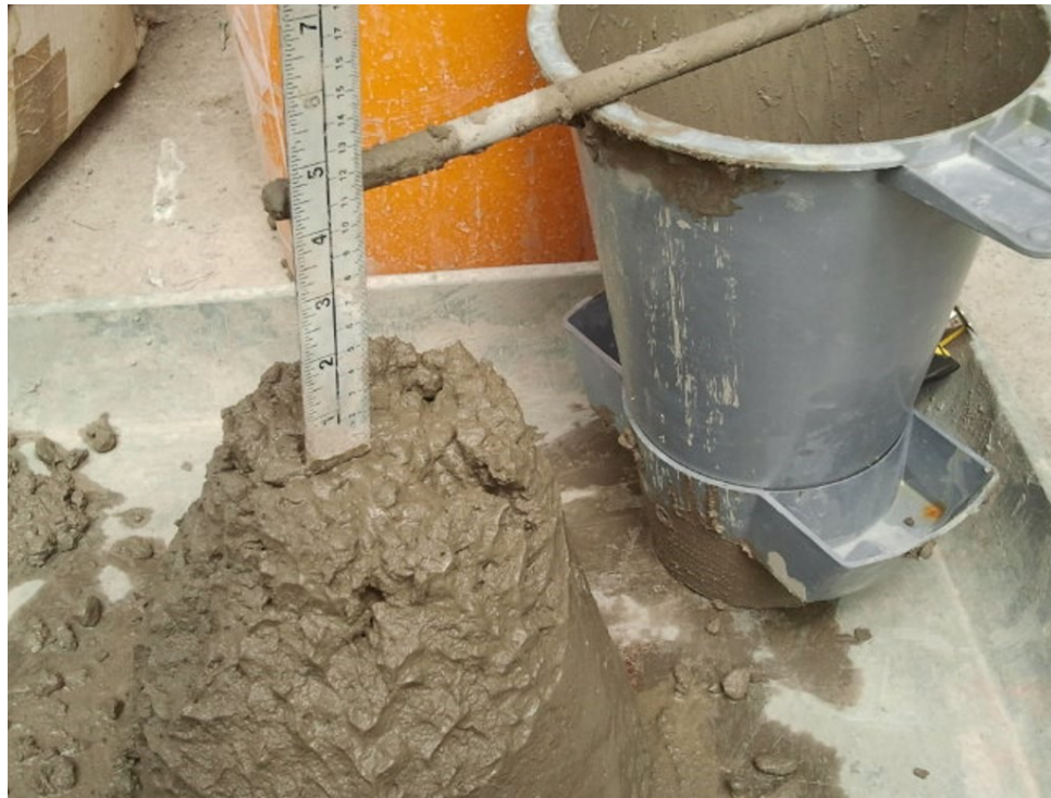
Figure 3-9: Slump test of concrete mix
