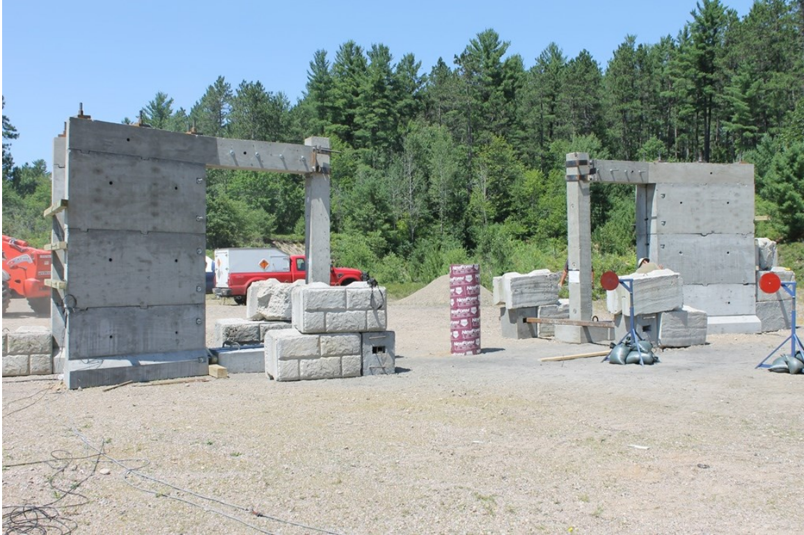
Figure 4-2: Photographs of columns (CONV-7 and SEIS-8) prior to explosion
