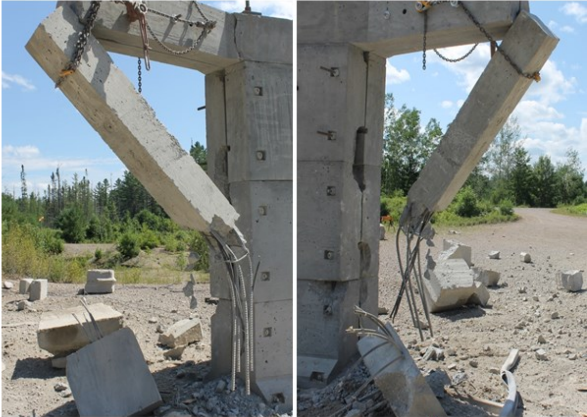
Figure 4-50: Post-test photograph of column CONV-2
