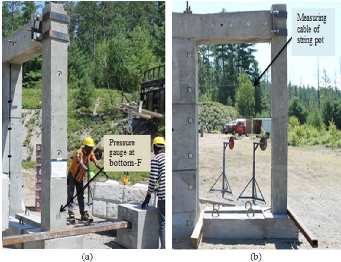
Figure 4-11: Photograph of Column CONV-7 showing; (a) pressure gauge location (b) measuring cable of string potentiometer at 2 m from the base of the column
