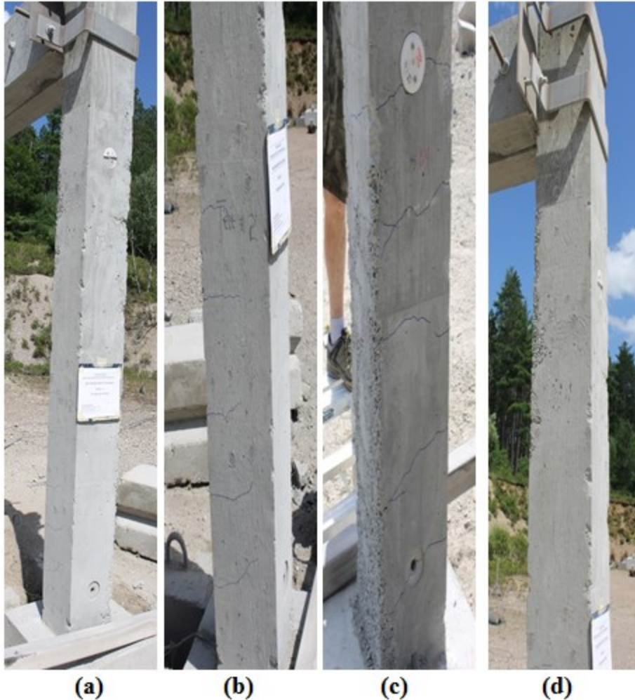
Figure 4-52: Post-test photograph of column SEIS-14 faces: (a) Front face, (b) Side face (right), (c) Back face, and (d) Side face (left)
