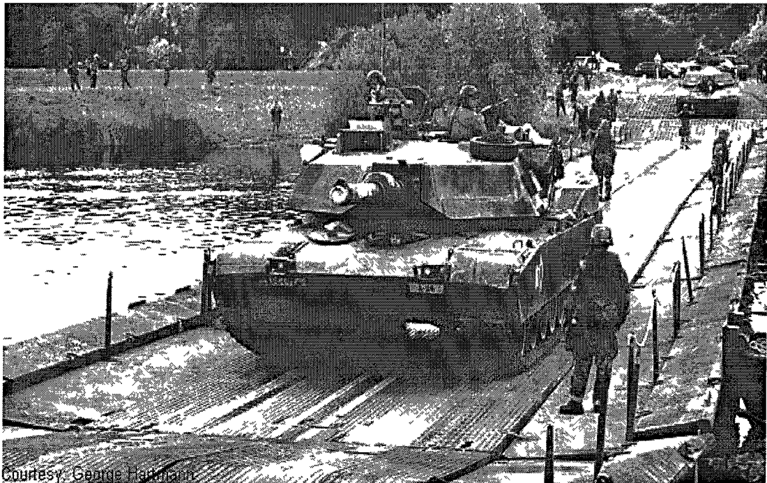
Figure 3.3 Ribbon bridge traversed by a tank concentric along the bridge centre line (defenselink.com)
