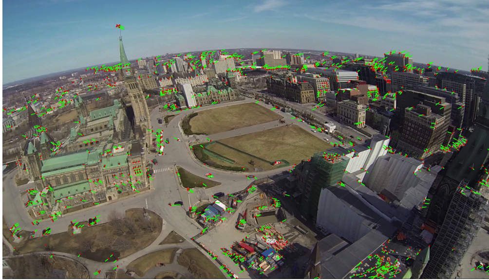
FIGURE 3.4: Visualization of distortion and desired correction. An exaggerated example of a distorted video frame from the parliament video, and lines showing how the image should be corrected.
