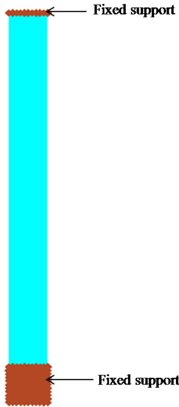
Figure 3-10: Fixed supports condition of RC column
