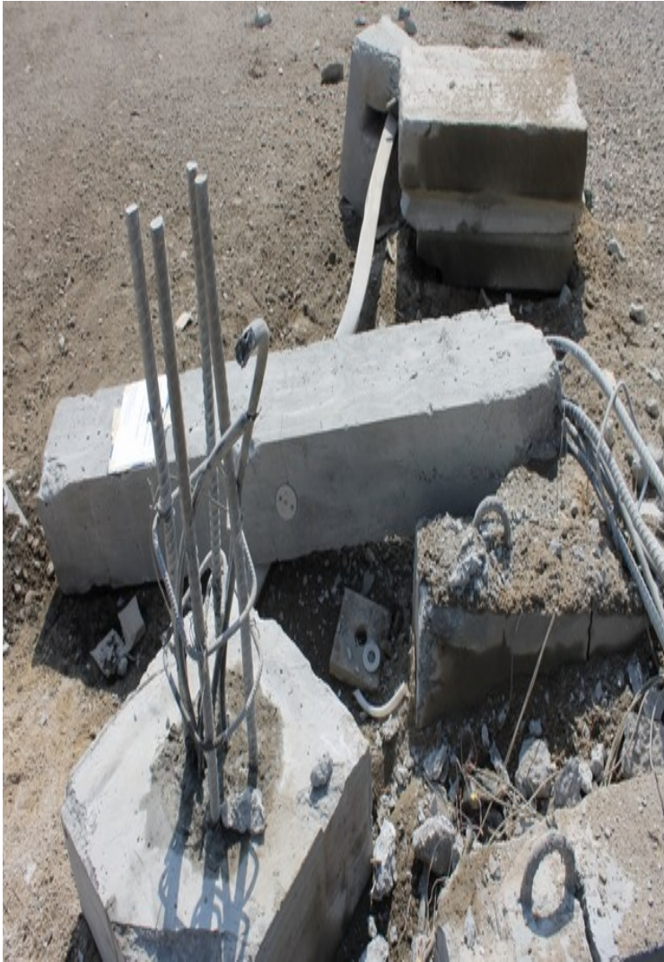
Figure 3-24: Visual display of the failed columns at standoff distance of 1.3 m
