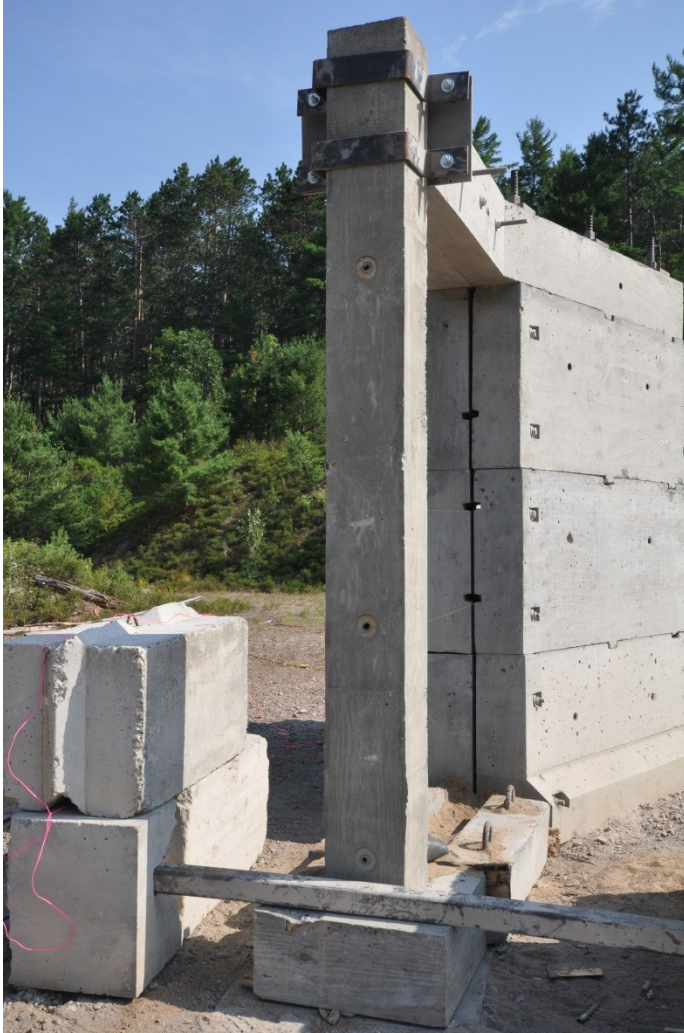
Figure 3-26: RC Colum on Site prior to testing
