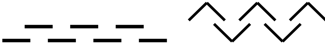
Figure 66: (a) Double-layer plate configuration, (b) Double-layer nested side-by-side angle configuration (Koger et al., 1975)
