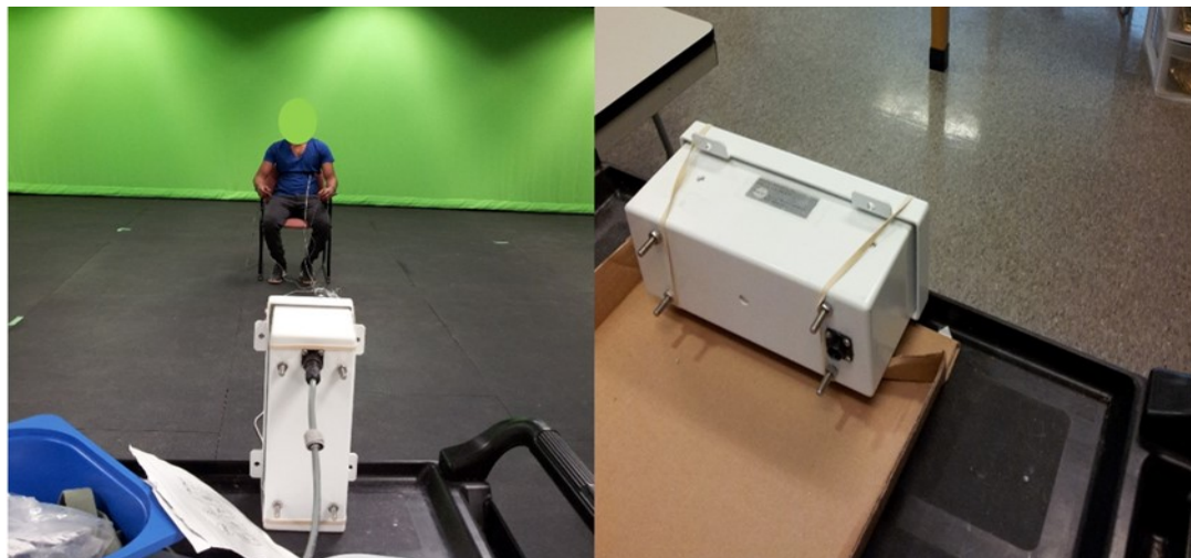
Figure 3.1 The SR12003 radar unit in its vertical orientation (left) and horizontal orientation (right).
