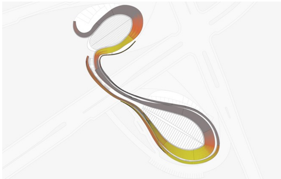
Figure 3.21: plan highlighting surfaces exposed to varying levels of irradiation, annually
