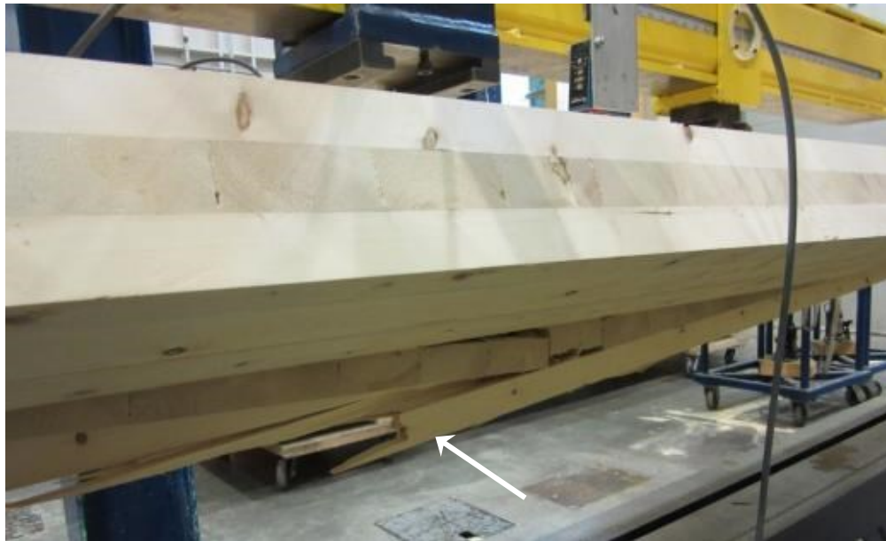
Figure 3.9 – Bending Test 2 failure mode (tension at lower laminations)
