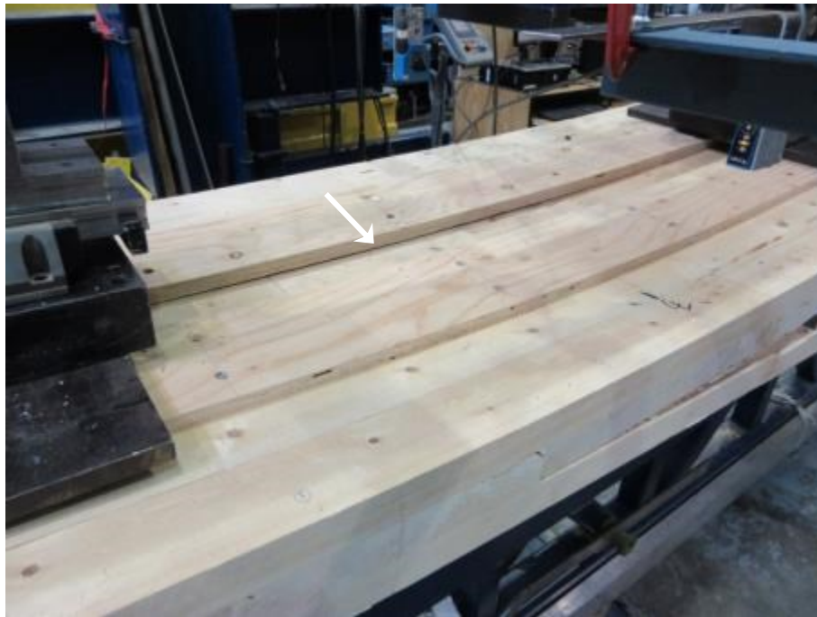
Figure 3.7 – Bending Test 1 plywood spline and fasteners after failure
