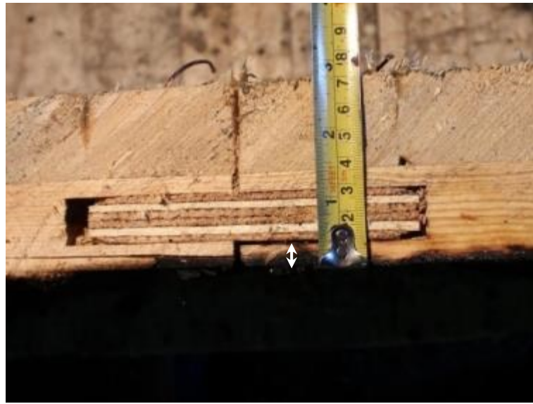
Figure 3.21 – Fire Test 1 residual cross-section after testing
