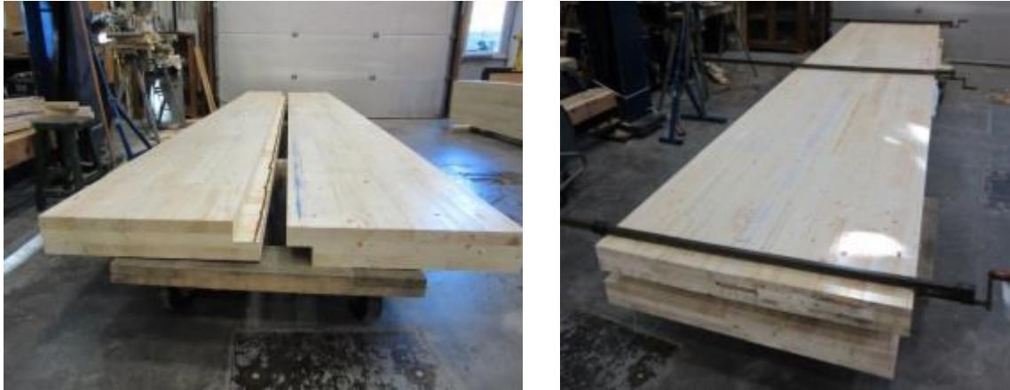
Figure 3.1 – CLT panels ready to assemble (left) and under side pressure by clamps (right)
