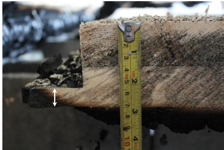
Figure 3.24 – Fire Test 2 residual cross-section after testing
