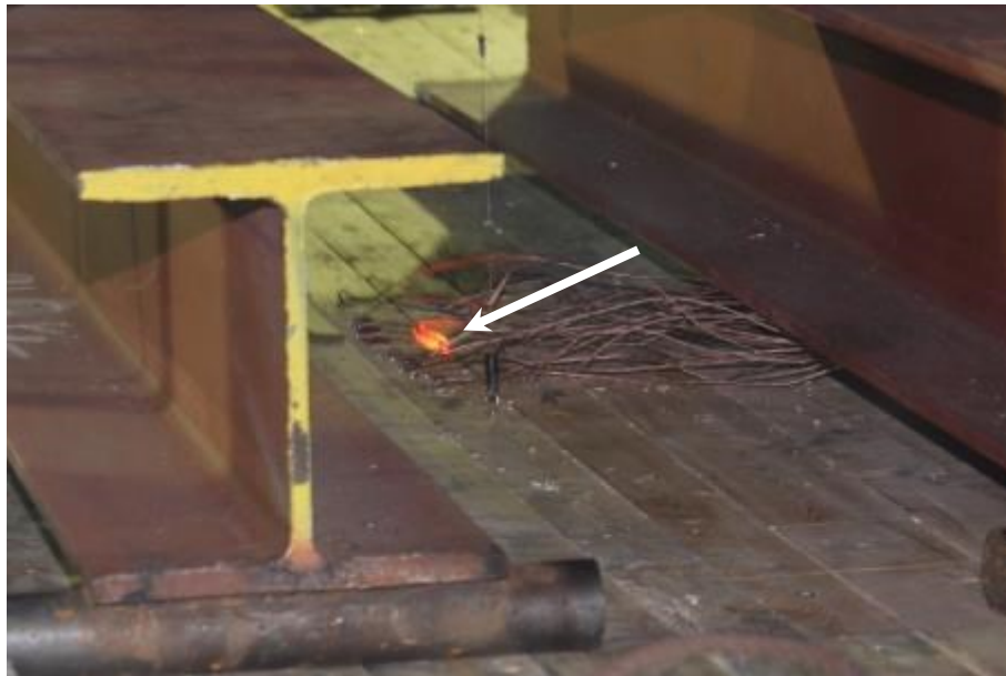
Figure 3.32 – Fire Test 5 failure (fire integrity) at 76 min
