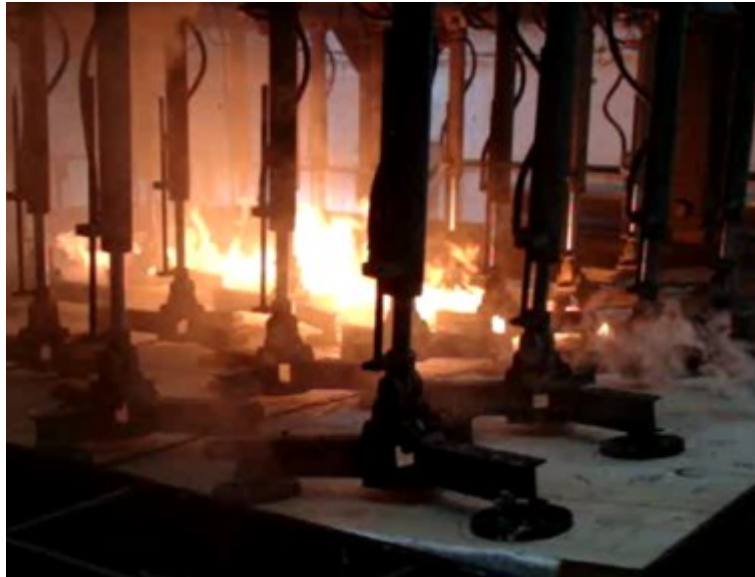
Figure 2.4 – CLT panel-to-panel fire integrity failure (flame-through) (credit: NRC/FPInnovations)
