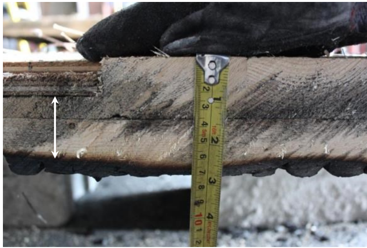
Figure 3.27 – Fire Test 3 residual cross-section after testing
