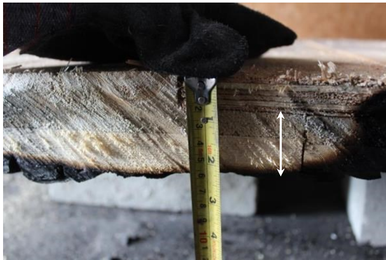
Figure 3.30 – Fire Test 4 residual cross-section after testing
