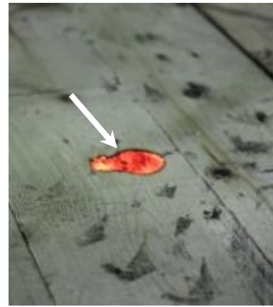
b) Close-up of the burn-through hole
