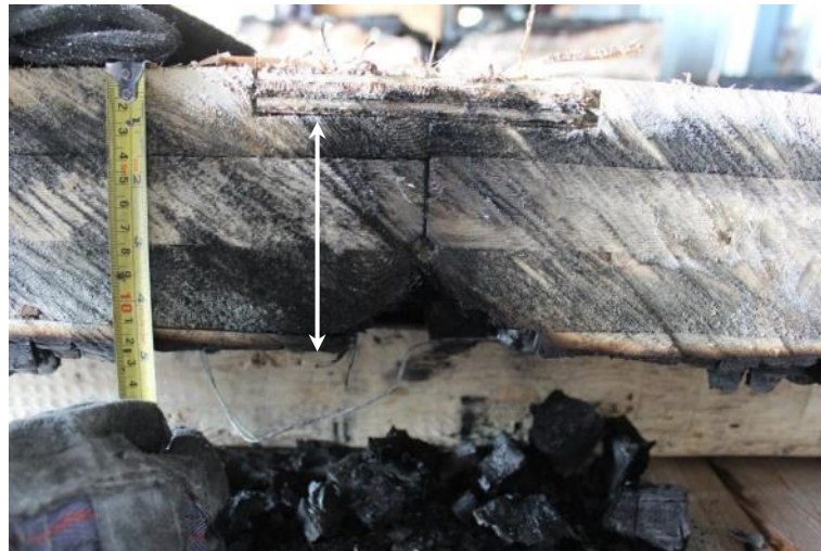
Figure 3.42 – Fire Test 8 residual cross-section after testing
