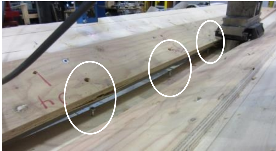
Figure 3.8 – Bending Test 2 failure mode (head pull-through of self-tapping screws)
