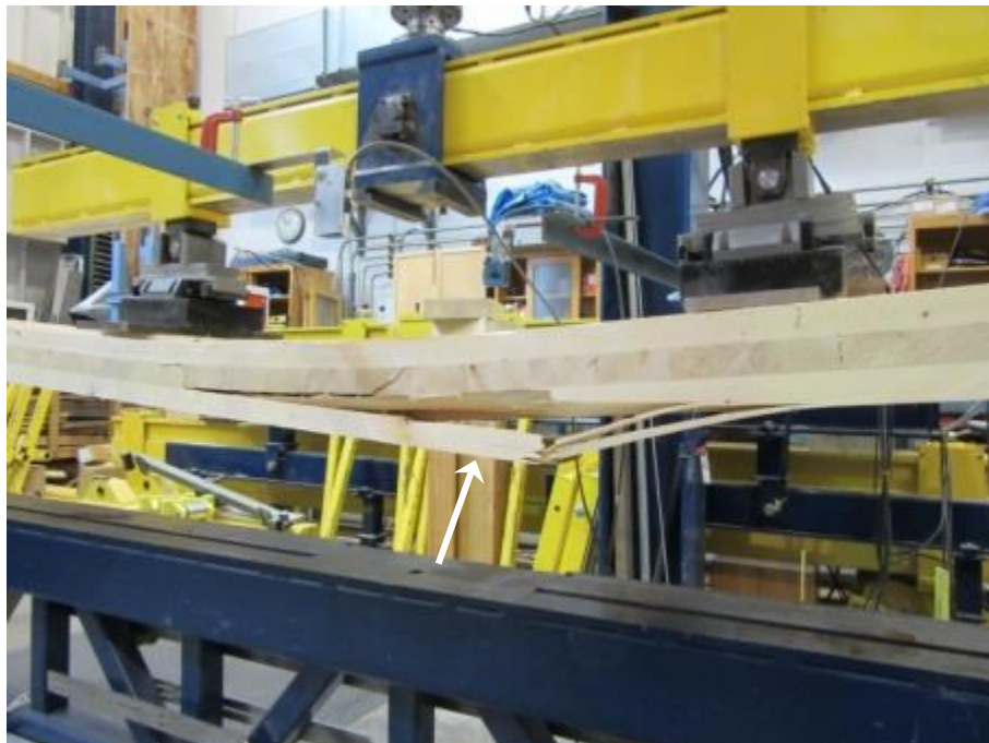
Figure 3.6 – Bending Test 1-retest failure mode
