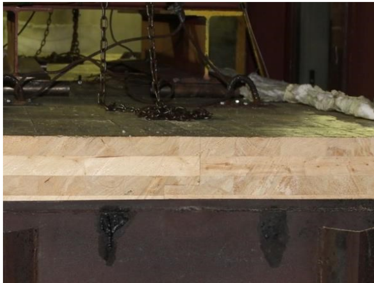
Figure 3.34 – Fire Test 6 specimen installed inside the furnace frame
