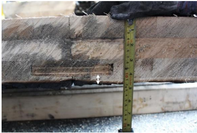
Figure 3.33 – Fire Test 5 residual cross-section after testing
