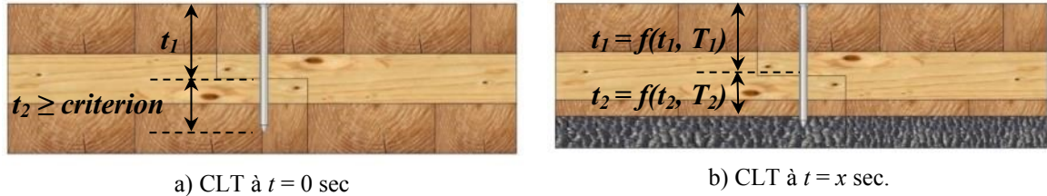
Figure 5.2 – Schematic of the coupled thermal-structural model
