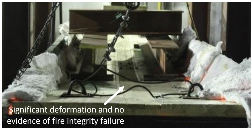
Figure 3.26 – Fire Test 3 after 54 min of fire exposure (no failure)
