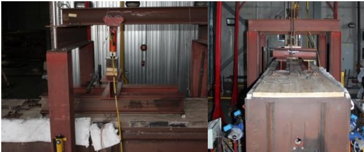
Figure 3.11 – Intermediate-scale test furnace at Carleton University
