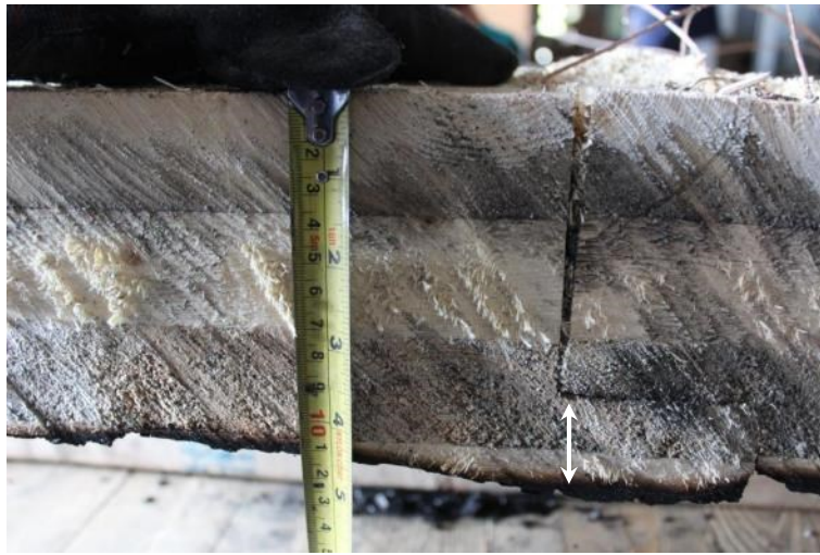
Figure 3.36 – Fire Test 6 residual cross-section after testing
