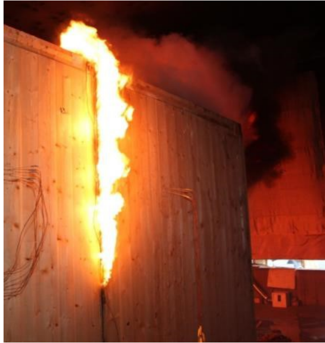
Figure 2.6 – Flaming through a half-lapped joint during a fire test by Medina [42]
