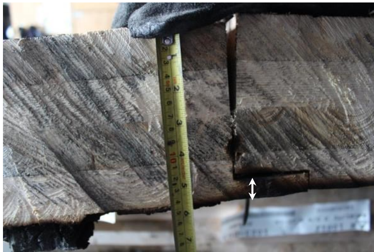
Figure 3.46 – Fire Test 9 residual cross-section after testing
