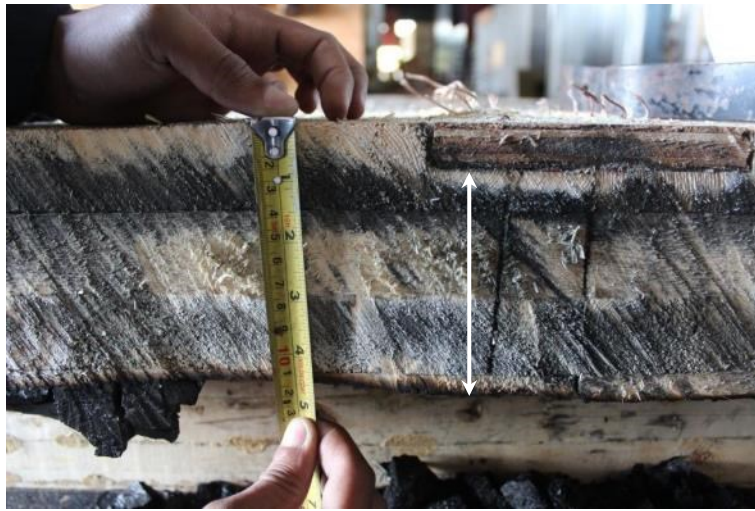
Figure 3.39 – Fire Test 7 residual cross-section after testing
