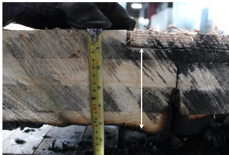
Figure 3.49 – Fire Test 10 residual cross-section after testing
