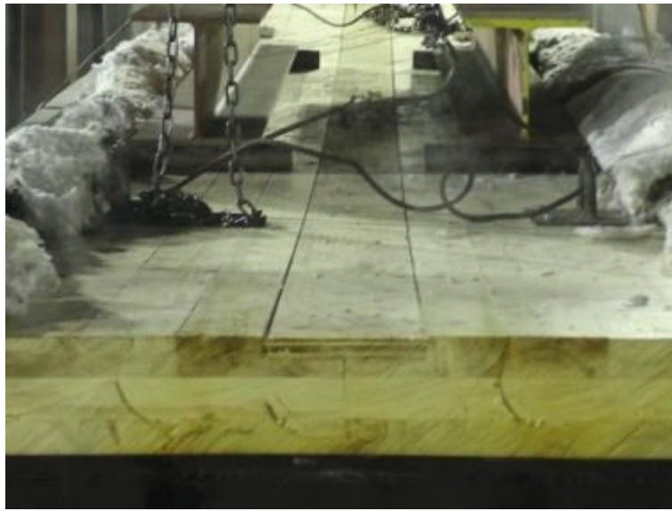
Figure 3.37 – Fire Test 7 specimen installed inside the furnace frame
