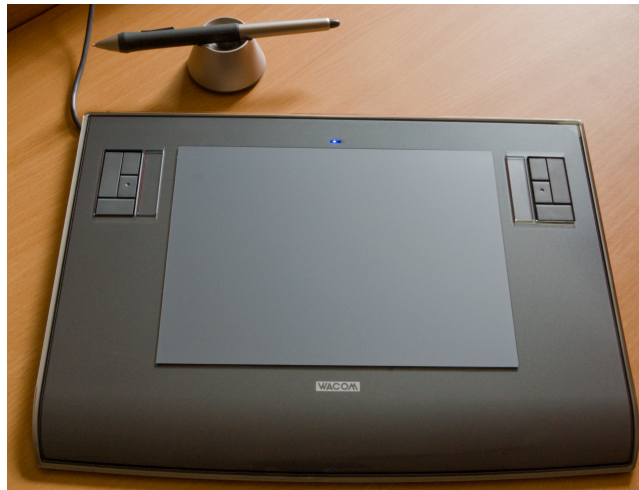
Figure 3.14: The Wacom Intuos 3, a popular graphic tablet, with its matching pen. The active area is the lighter rectangle in the center. Image reproduced from [55].
