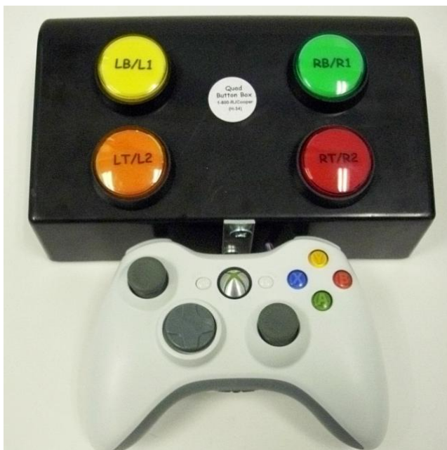
Figure 3.2: The Quad Button Box and mounted Xbox 360 controller. Image reproduced from [160]
