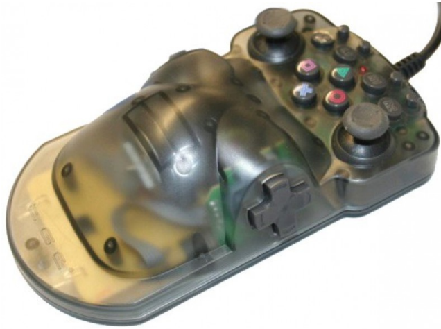
Figure 3.8: The One-Handed Ergonomic Palm Game Controller. Image reproduced from [39].
