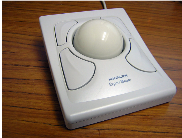
Figure 3.16: The Kensington Expert Mouse, a trackball. The physical ball used is a standard billiard ball. Image reproduced from [173].
