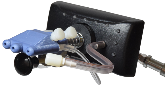
Figure 3.1: The Original QuadStick. Image reproduced from [152].
