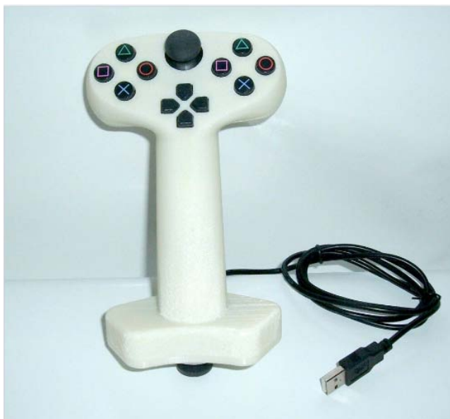
Figure 3.10: The ORTHOS One Handed Handset. This image shows the USB version. Image reproduced from [105].
