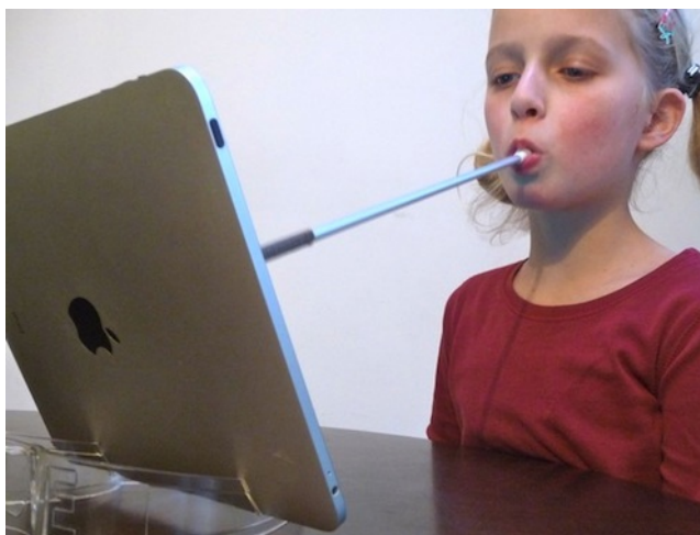
Figure 3.26: A girl using a mouth stick to operate an iPad. Image reproduced from [37].
