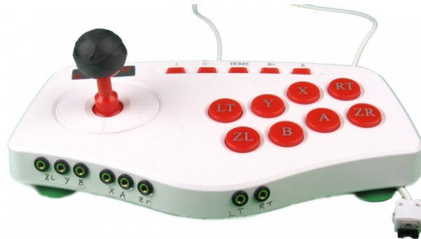
Figure 3.6: The Nintendo Wii Switch Enabled Classic Arcade Controller. Image reproduced from [38].
