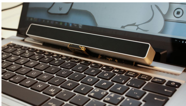
Figure 3.18: The Eye Tribe, a consumer priced eye-tracking device, mounted to the screen of a laptop computer. Image reproduced from [175].
