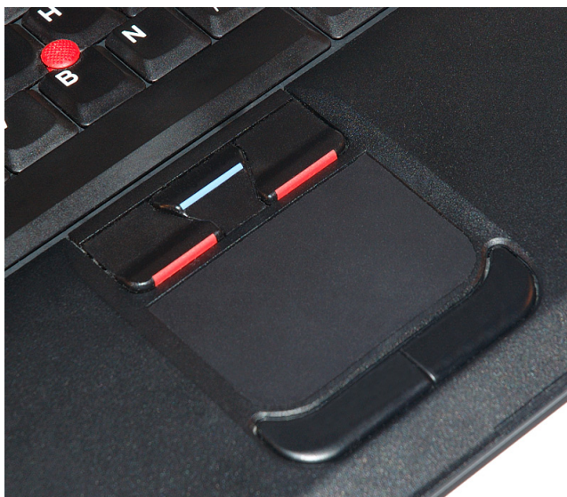
Figure 3.12: The trackpad from an IBM ThinkPad laptop computer. Image reproduced from [93]
