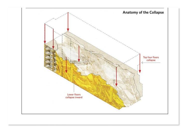
This picture reveals the process of the collapse. The top four floors (9th floor, under construction; 8th floor, New Wave; 7th floor, New Wave; and 6th floor, Phantom Tac) collapsed, which ultimately leveled the building.
